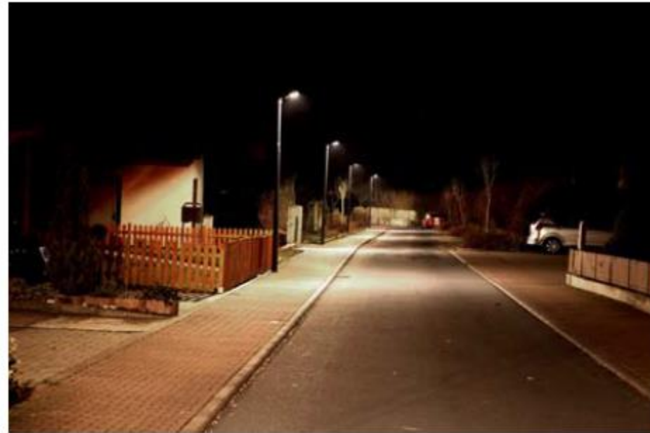
Fig. 4 b: 3000K LED Lighting Used after Replacement
